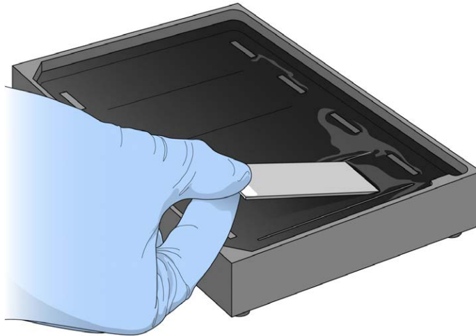
Figure 42 Placing BeadChip into Black Frame on Alignment Fixture
