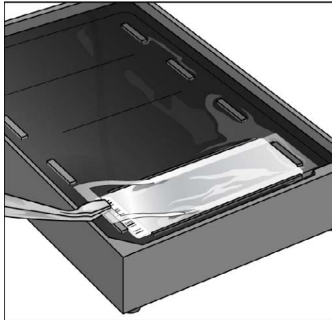
Figure 103 Placing Clear Plastic Spacer onto BeadChip
