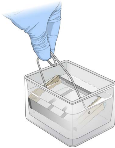
Figure 98 Wash Rack in Wash Dish Containing PB1
