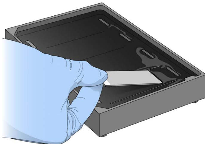
Figure 102 Placing BeadChip into Black Frame on Alignment Fixture
