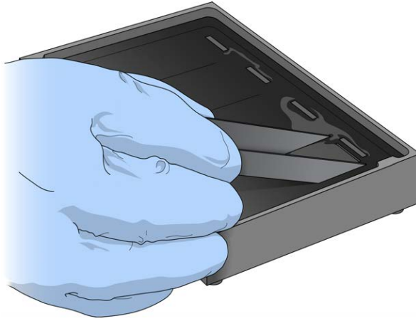
Figure 41 Placing Black Frames into BeadChip Alignment Fixture
