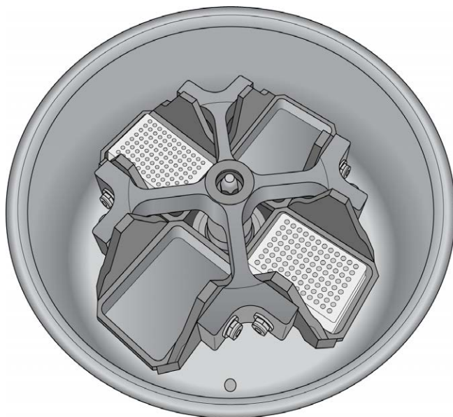
Figure 16 Sealed MSA5 Plate and Plate of Equal Balance in Centrifuge
