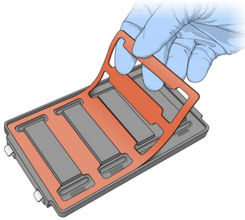
Figure 22 Placing Gasket into Hyb Chamber
