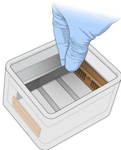
Figure 100 Submerging BeadChips in Wash Dish Containing PB1
