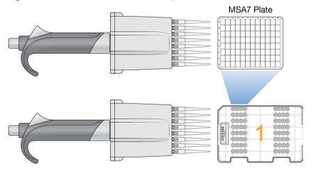
Figure 7 Correct and Incorrect Orientation of a Micropipette Tip in the XT Tip Guide
