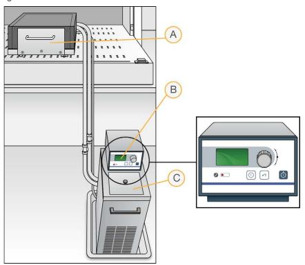
Figure 30 Water Circulator Connected to Chamber Rack
