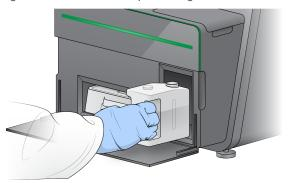
2 To prevent spills when carrying the spent reagents bottle, seal the bottle opening with the threaded cap.
