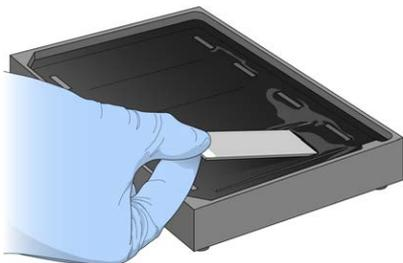
5. Place a **clear** spacer onto the top of each BeadChip. Use the alignment fixture grooves to guide the spacers into position.
