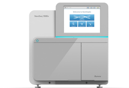
Figure 6: The NextSeq 550Dx System—Developed under design control and manufactured following good manufacturing practice (GMP) guidelines, the NextSeq 550Dx System (in Dx mode) supports a fully automated TSO Comprehensive (EU) workflow from sequencing through final clinical report generation.
